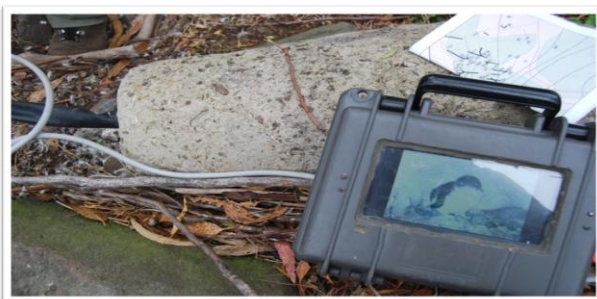
Figure 2.11. Infra-red burrowscope equipped with a camera showing an igloo occupied by a moulting little penguin.
