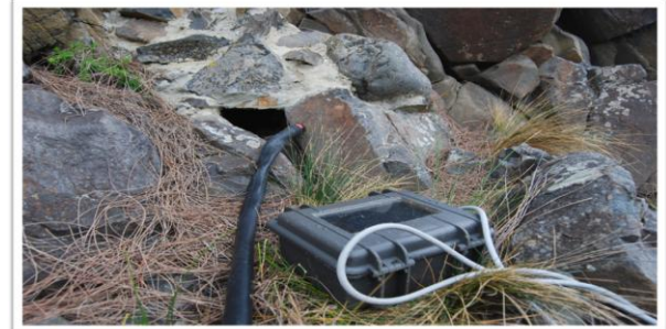
Figure 2.12. The use of infra-red burrowscope suits any type of nest hard to access directly.
